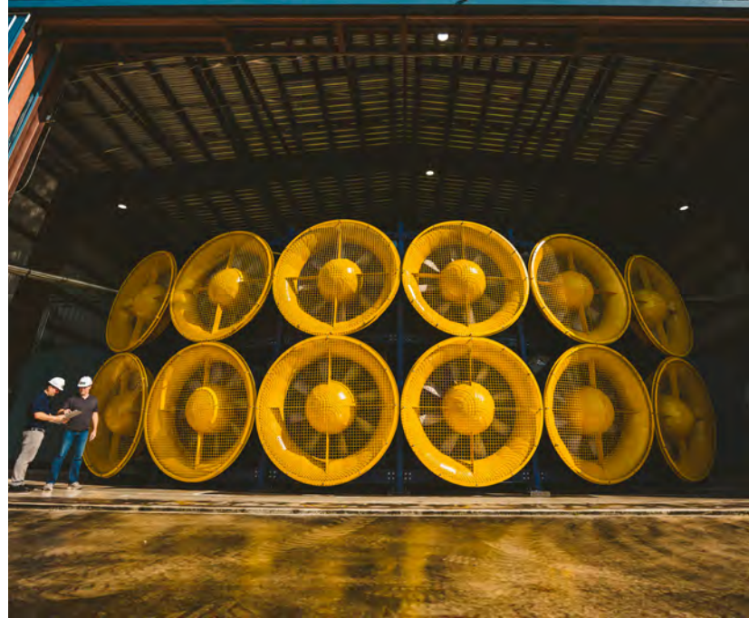
The NSF-NHERI Wall of Wind at Florida International University. Photo credit: Florida International University
